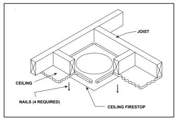
Figure 10.15 Ceiling Firestop (Ceiling Side)
